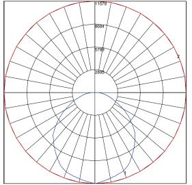
Maximum Candela = 11578 Located At Horizontal Angle = 0, Vertical Angle = 0 # 1 - Vertical Plane Through Horizontal Angles (0 - 180) (Through Max. Cd.) # 2 - Horizontal Cone Through Vertical Angle (0) (Through Max. Cd.)
