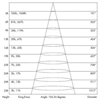
Note: The curves indicate the illuminated area and the average illumination when the luminaire is at different distances.
